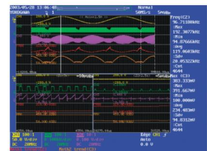
You can measure commercial power supply voltage and switching voltage/current in active power correction circuits, and also plot fluctuations in switching frequency and switching current.
