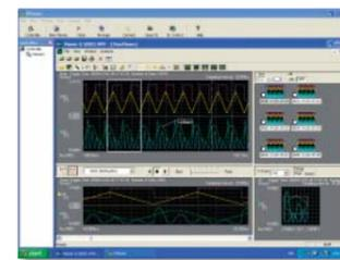
Xviewer is a PC software application designed to work with Yokogawa's DL series digital oscilloscopes and the DL750 series ScopeCorders. Xviewer allows you to display DL-acquired waveform data (using the "Viewer" function), perform file transfers, and control DL series instruments remotely.
