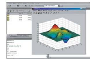
The MATLAB tool kit for the DL series is a plug-in for MATLAB software. The toolkit can be used to control supported DL series instruments using MATLAB or to acquire data from a DL series instrument for use in MATLAB via a communication interface (GP-IB, USB, Ethernet).
