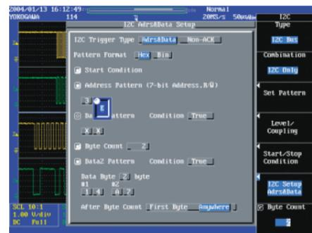
I<sup>2</sup>C Address and Data Trigger Setup Menu
