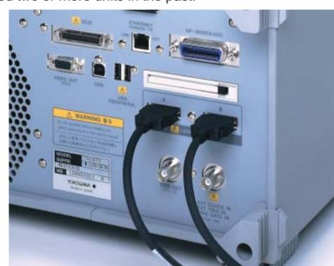
Example of Logic Probe Connection
