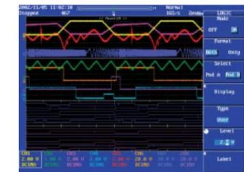
8-channel analog and 16-bit logic display
