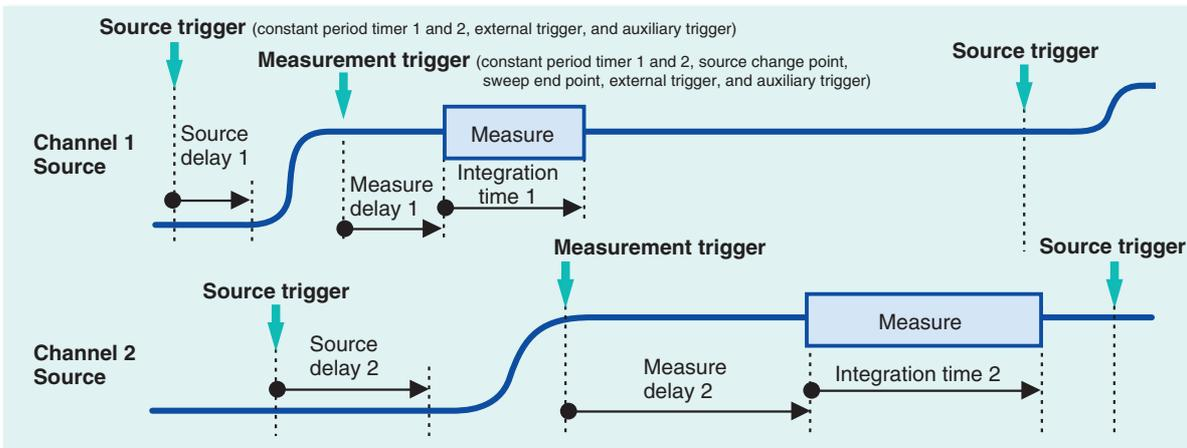
Asynchronous Operation of Source and Measure
