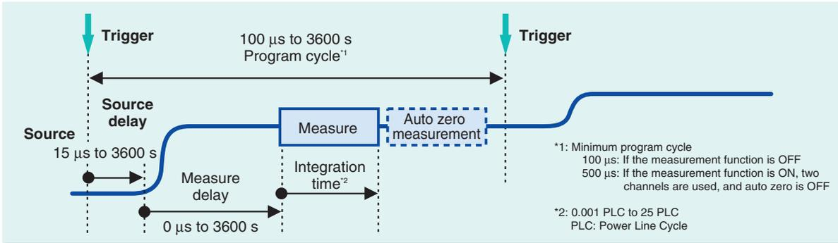
Timing Settings Using Various Trigger Sources
