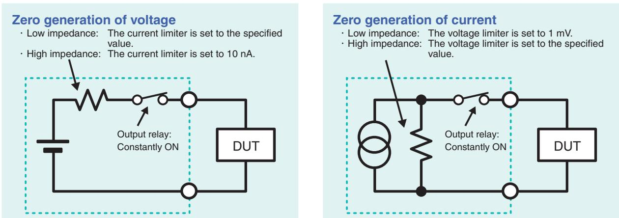
Measurement of the Static Characteristics of Three-Terminal Semiconductor Devices (Transistors, FETs, etc.)
